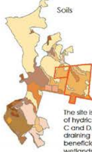
The site is composed of hydric soil groups C and D. These are poorly draining soils which can be beneficial for constructed wetlands.
