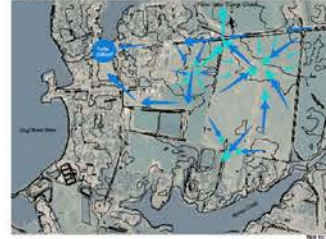
The proposed constructed wetlands are to help reduce the amount of water that contributes to the creation of "Lake Oxford" during storm events. Filling the existing outfall to Town Creek will allow for redirecting the water away from "Lake Oxford".
