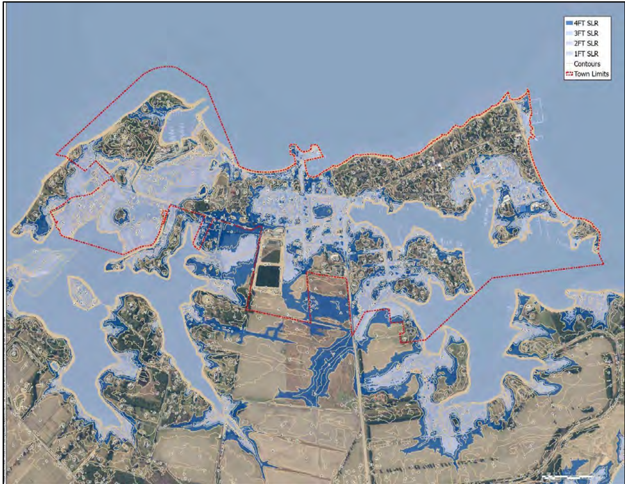
Fig. IV.B.3. Inundation at elevation 4.0' due to sea level rise or storm surge for Oxford, MD.
