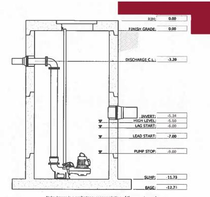
Note: Image is a preliminary representation of the pumping system. Elevations shown are the primary factors used for sizing the wet well.
